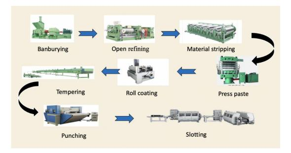
Figure 2: The production process in selected stages.
